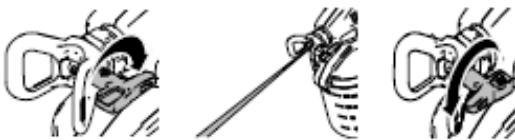
3. Release the trigger safety lock and press the on/off switch for approx. 10 seconds to ventilate the pump. Release the trigger and place the ventilation/discharge valve downwards in the spray position.
