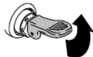
2. Place the ventilation/discharge valve in the upwards position (UP) and hold down the trigger for 10 seconds.
