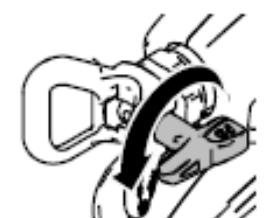
7. Once the clog has been removed, activate the trigger safety lock and turn the nozzle back to the spray position.
