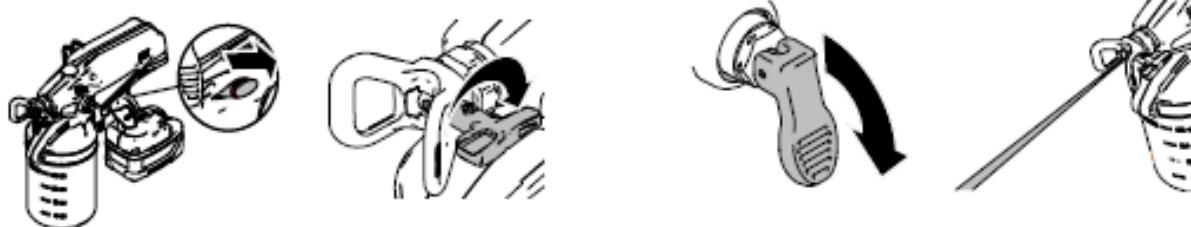
8. Release the trigger safety lock, turn the nozzler to the cleaning position, and pull the trigger for approx. 5 seconds to ventilate the spray device.
