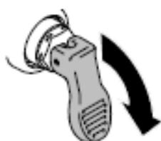
3. After, place the ventilation/discharge valve downwards into the spray position (DOWN).
