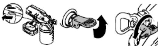
3. Direct the spray device into an empty container, unlock the trigger safety lock and switch the ventilation/discharge valve downwards into the spray position. Press the trigger to remove the clog.
