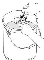
11. Remove the material hopper and dispose of any used rinsing fluid correctly.
