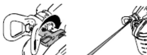
4. Turn the nozzle into the cleaning position, direct it into a waste bin, and then press the pistol's trigger.
