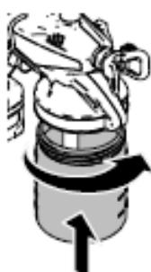
1. Fill the material hopper with water and screw it onto the spray device.
